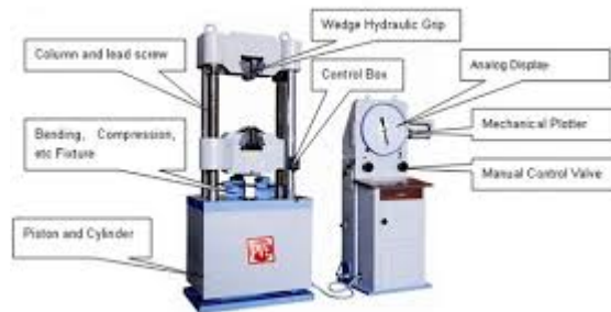
UNIVERSAL TESTING MACHINE(UTM).
