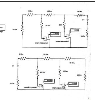
Current through Load Resistor(R<sub>L</sub>) 200 Ohms :
