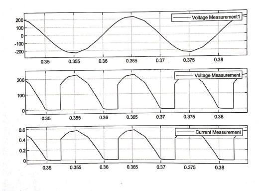
**<u>CONCLUSION:</u>** From the above experiments we able to draw the single phase full bridge controlled rectifier by using simulink.
