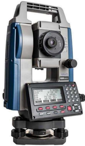
Fig: An EDM fitted on Total Station
