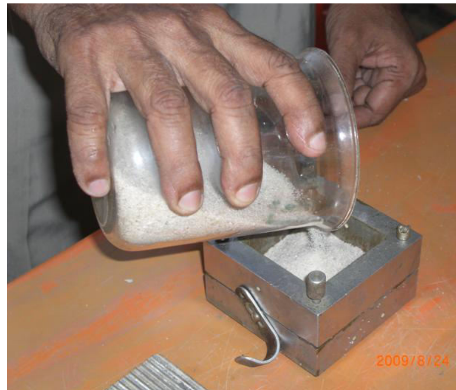
Preparation of a sand specimen
