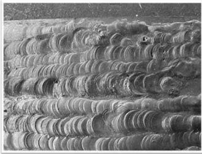
Figure 7.23 unacceptable weld profiles
