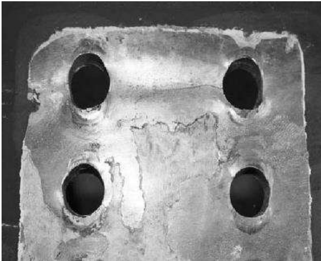
Figure 10.16 Bearing failure of plates
